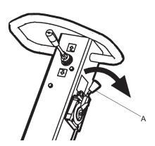
2. Set the throttle control (A) in stop position.
