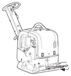
Check the screws and nuts on the safety straps, if necessary tighten or replace.
