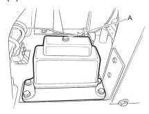
2. Fill up with hydraulic oil if necessary, see chapter "Hydraulic system, changing the hydraulic oil".
