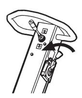
3. Pull out the starter rope until it resists. Release the handle so the starter rope goes back again, and then pull the starter rope until the engine starts.
