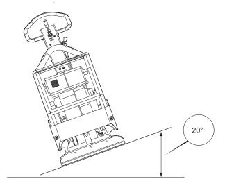
The tilting angle is measured on a hard level surface with the machine stationary. Vibration switched OFF and all tanks full.
