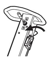
Close the choke valve if the engine is cold. If the engine is warm or the ambient temperature is high, close the choke valve halfway or leave it open.
