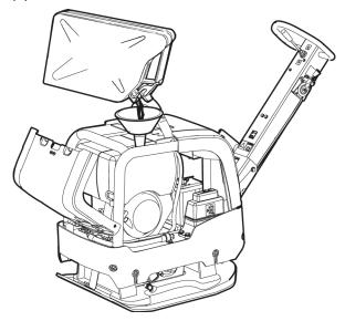
4. Never overfill the tank. Due to the movement of the fuel within the tank, it is possible to have fuel at a higher level than the tank cap, which can lead to a spillage of fuel if the tank cap is opened. This can be avoided by only opening the tank cap, when the machine is tilted and the tank cap is at the fuel tank's highest point.
