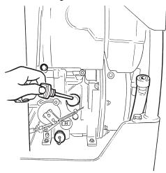
2. Set the throttle control (A) to half revs.
