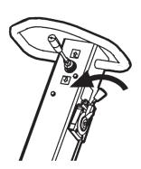
Turn the ignition key to ignition position 1. The control lamps for charging and oil pressure light up.
