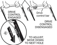
Over time, the drive control system may become "loose", resulting in decreased speed. There are holes in the drive control housing to increase tension on the drive cable. Proceed as follows:
