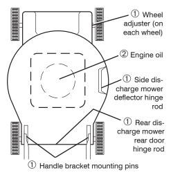
(1) Spray lubricant 2 See "ENGINE" in Maintenance section.
