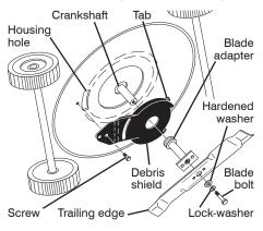
Use a wood block between blade and mower housing to prevent blade from turning when removing blade bolt.
