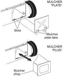
MULCHER PLUG BUILT INTO REAR DOOR
