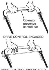
DRIVE CONTROL DISENGAGED
