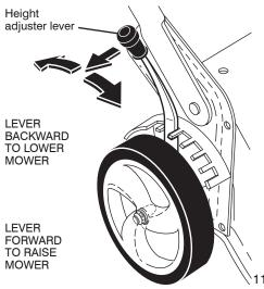
"THREE POINT" ADJUSTMENT (18" (45cm) HI-VAC MODELS ONLY) Both rear wheels are adjusted by a single lever on the left rear wheel.
