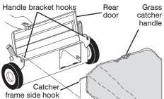
For DOOR PIVOT PIN mounted catcher, place the grass catcher frame hooks onto the door pivot pins.
