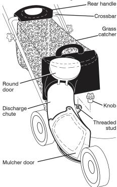
2. Open mulcher door and insert tabs of discharge chute into hinge bracket opening and position rear of chute over threaded stud.
