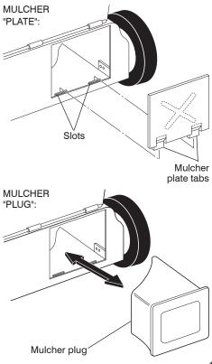
MULCHER PLUG BUILT INTO REAR DOOR
