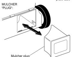
MULCHER PLUG BUILT INTO REAR DOOR
